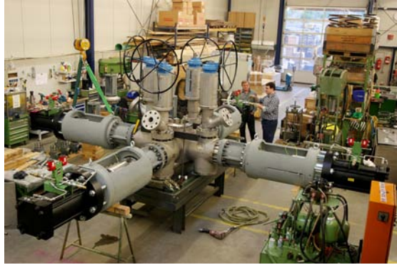
SchuF Fetterolf has built the largest and most advanced diverter and control valve assembly used in the world. It is installed at the Shenhua coal liquefaction plant in the world’s only full scale to coal to liquid fuel plant.
